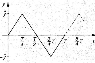
$$y(t) = \frac{8\hat{y}}{\pi^2} \left( \frac{1}{1^2} \cdot \sin(\omega_0 t) - \frac{1}{3^2} \cdot \sin(3\omega_0 t) + \frac{1}{5^2} \cdot \sin(5\omega_0 t) - + \dots \right)$$
