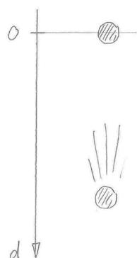
Distance  $d$  after time  $t$ :  $d = \frac{1}{2}gt^2$  ( $g$  = gravity field strength)
